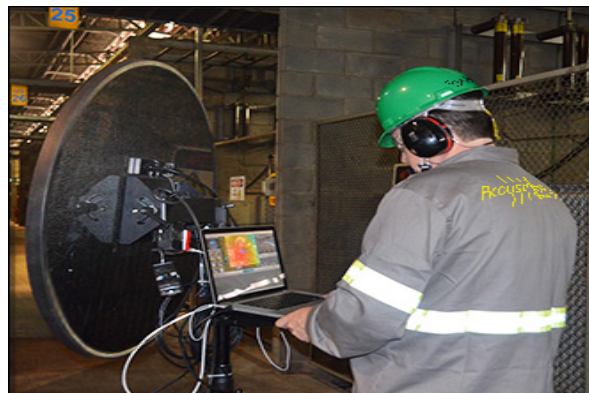
ARTVIS PINPOINTS NOISE SOURCE in 110dB AREA
