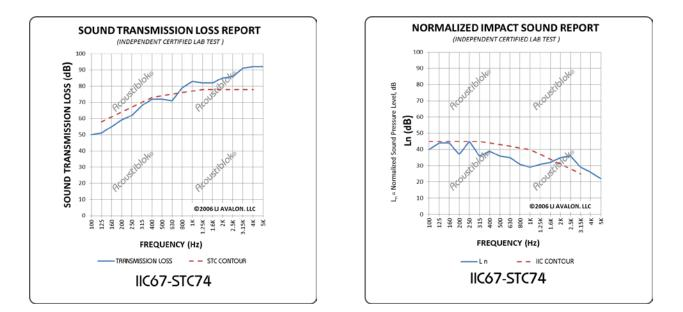
Independent testing services have rated this floor configuration with an IIC67 and an STC74.
