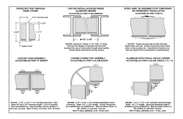
Panels are designed to be mounted vertically. If panels are to be mounted at an angle, (with perforation on the downside) Acoustiblok highly recommends sealing the solid aluminum to the frame of the panel with the Acoustiblok FCA10 adhesive and also seal up any drain holes in the frame which may be on the top side, leaving the drain holes on the bottom side open.
